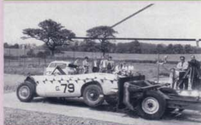
BGT Rear impact trolley (same weight as car).
