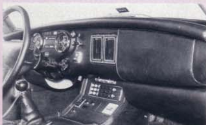
SSV1 Airbag & Knee protection mounting collapsing column- impact sensor-under knee roll & British Leyland Automatic start "Test" unit.
