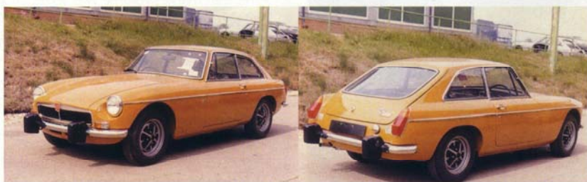
1st Production B GT Sabrina energy absorbing bumpers 5mph barrier compliance.
