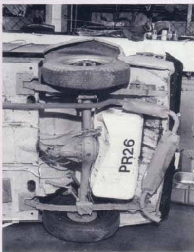
Underside of MGB after rear impact showing damage to fuel tank – possible puncture of tank on original type handbrake "swingle tree".
