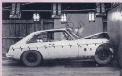
B GT at point of 30mph + impact taken at MIRA.
