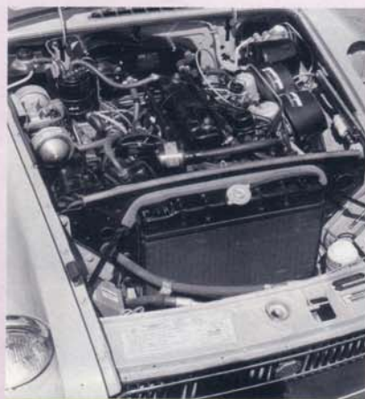
SSV1 Underbonnet – showing suspension control and roll/ride levelling units.
