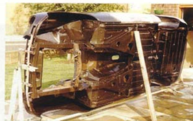
MGC Floor pan showing unique triangular box sections
