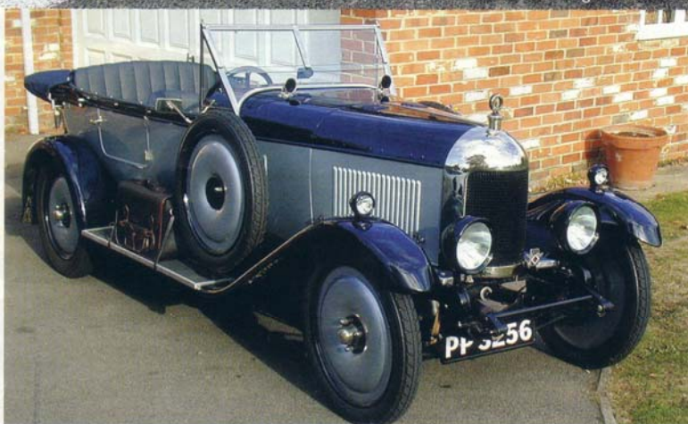
A 14/28 'Bullnose' Super Sports, Four-Seat Tourer. With its raked windscreen, lowered suspension, disc wheels and altered steering arrangement, these vehicles supplied good handling and a sporty feel that endeared them to young bucks of the 1920s.
