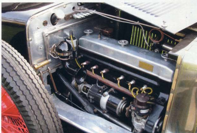
The engine bay of an Mk I 18/80. All of the components are easy to reach for adjustment, the OHV engine is easy to service and with the auxiliary petrol tank filler (unseen in this image) means that you can carry a backup supply of both fluids with ease.
