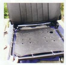
together — working from top to bottom. Photo II. Once complete, apply books, etc, to weigh the cover down to ensure the two don't pull apart.
