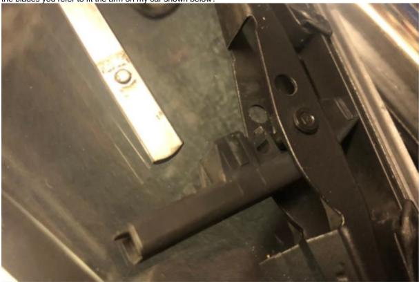
**Tony Lake** replied "Yes it is the same as mine. Because the new blade assembly is designed for a hook shaped wiper arm you must remove the plastic pivot that fits on the hook so that you end up with just a wiper blade. Then when you remove your old wiper assembly you have to reuse the plastic pivot from the old wiper. It will be a lot clearer when you get hold of the new bits. Make sure you get **SP13**, there are other similar designations but I know SP13 fits.
